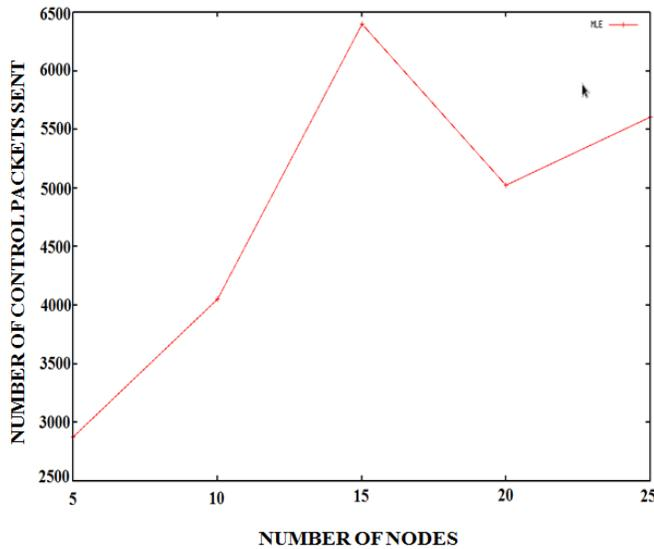
Fig. 3: Number of Control Packets Sent w.r.t Number of Node's
