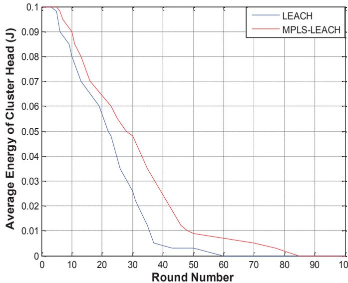
Figure 3: Traditional LEACH versus MPLS based LEACH.
