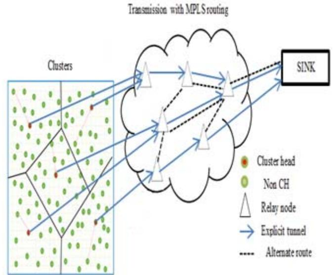
Figure 2: Illustration of MPLS based LEACH protocol
