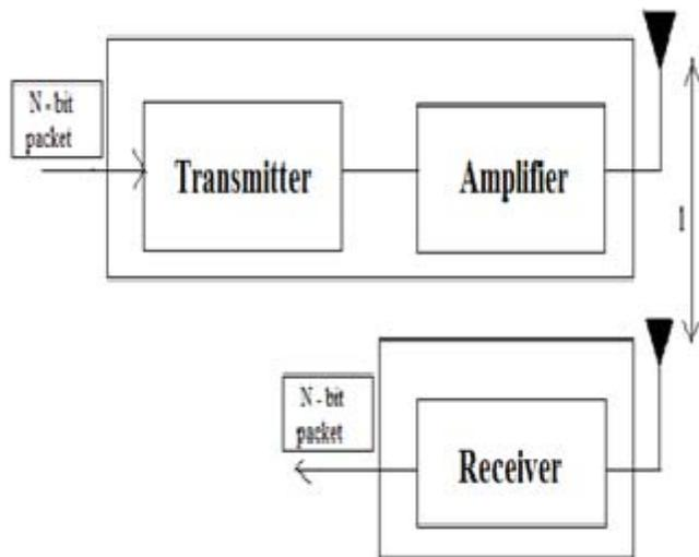
Figure 1: Block diagram of radio model
