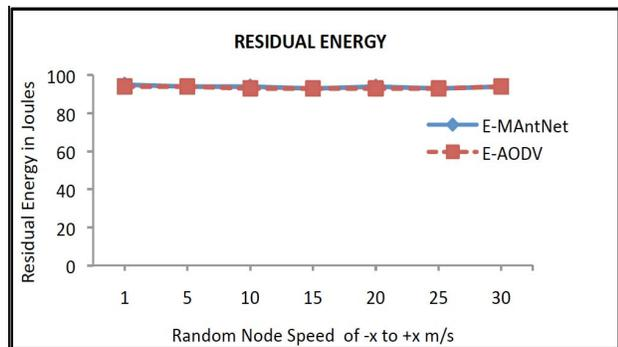
Fig. 11: E-MAntNet vs. E-AODV in terms of RE under varying RMS speed.
