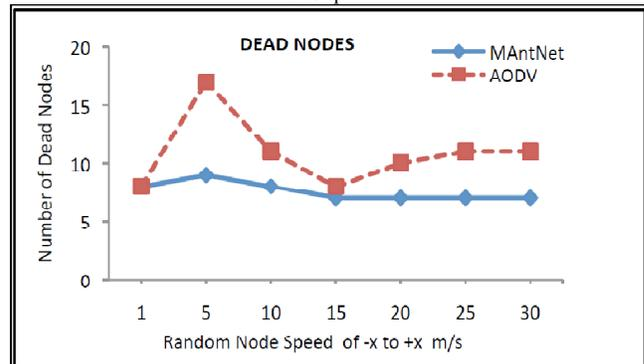
Fig. 14: MAntNet vs. AODV in terms of number of DN, under varying RMS speed
