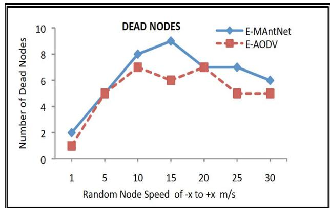
Fig. 13: E-MAntNet vs. E-AODV in terms of number of DN, under varying RMS speed
